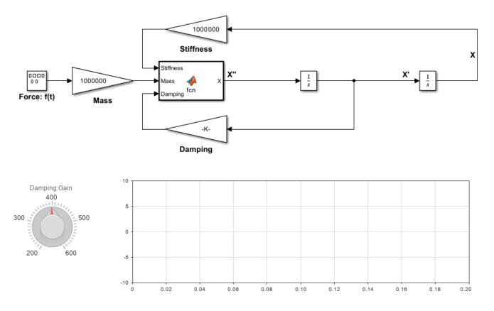
The model implements a second-order physical system called an ideal mass-spring-damper system. Gain blocks represent components of the system equation: Mass, Stiffness, and Damping. The equation for the system is mX'' + cX' + kX = f(t).
